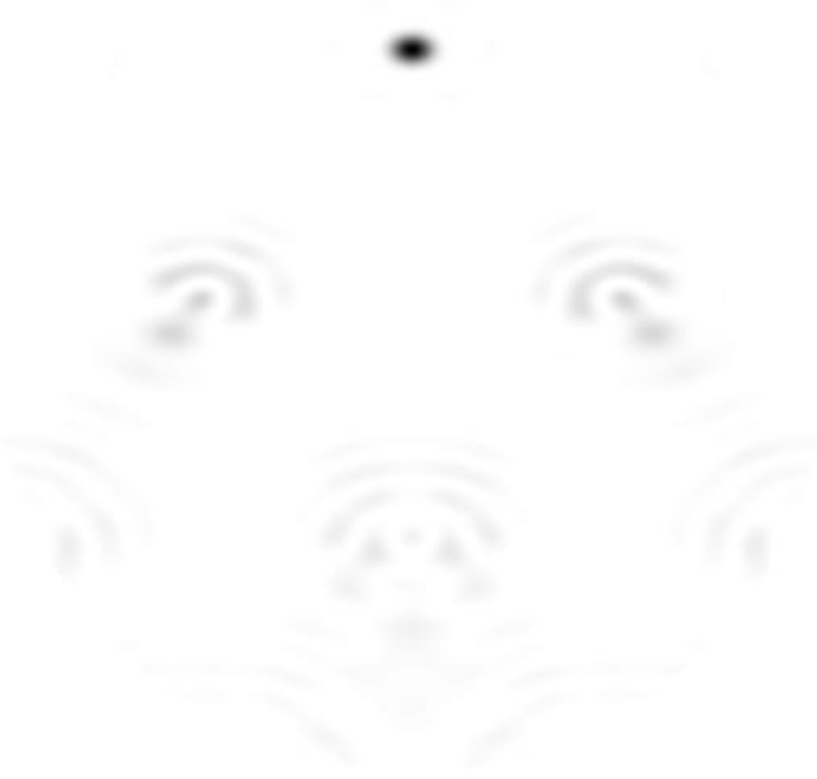
Fig. 7 Polar projection of beam pattern for the array populated with isotropic receivers. This shows the worst case side lobes, which occurs at the shortest wavelength, i.e. 200 Mhz. A spacing of 1.75m projected on the NCP was used. The small residual side lobes are further suppressed by 20 dB due to the primary beam of each log periodic. The horizontal scale is 180 degrees, the vertical scale is 120 degrees. The primary beam is actually round when viewed from the NCP.
