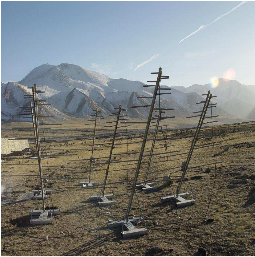
Fig. 1 Prototype pod layout. The pod has an element separation between neighboring antennae of 2m when projected onto the NCP. The elements were summed with the appropriate delay lines to place the main lobe on the NCP.
